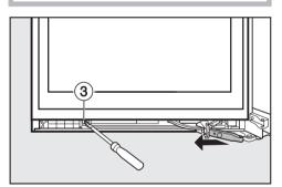
Screw the spacer and the soft-close mechanism together securely using screw (3).
